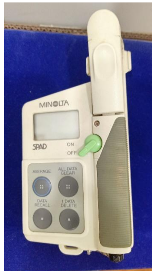
Figure 10. Leaf chlorophyll content measuring SPAD meter.
